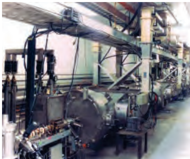
[Above]: Inside the accelerator, the electron beam circles the tunnel up to five times, gaining energy with each orbit. By the fifth time around, in a journey that has taken mere millionths of a second, each electron has attained an energy of 6 billion electron volts. [Left]: In a laboratory room above the free-electron laser [FEL], William and Mary Associate Professor of Applied Science Brian Holloway makes adjustments to equipment that uses laser light for making nanotubes.
