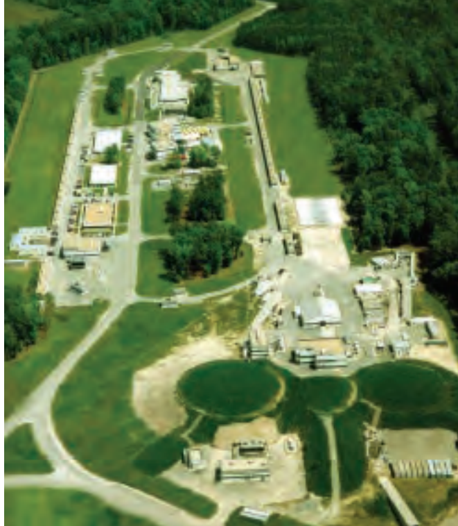
The service buildings shown in this aerial photo trace out the 7/8-mile racetrack shape of the accelerator tunnel, located 25 feet underground. Data-gathering takes place in each of three underground experiment halls, whose domed roofs are covered by vegetation and are visible in the lower right.
